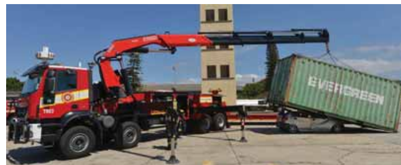
Heavy lifting: The Fire and Rescue Service's new R7,7 million Iveco Trakker 8x4 heavy-duty rescue recovery vehicle has a Fassi F660 crane with a lift capacity of 56,8 m and a maximum reach of 30,4 m. It also has two Waldon 30-ton hydraulic winches, each with a 60 m cable.
